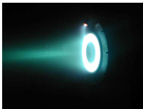
Figure 1.1. Hall Effect Thruster [1]
