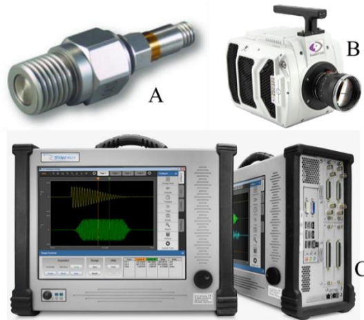
Figure 3.5: PCB Flush Mount Sensor(A), Phantom v2012 Camera(B), and Hi-Techniques Data Acquisition System(C) [65] [66] [67]
