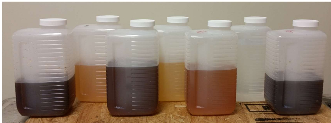
Figure B.1. Green roof runoff collected after Rainfall Event #2.
