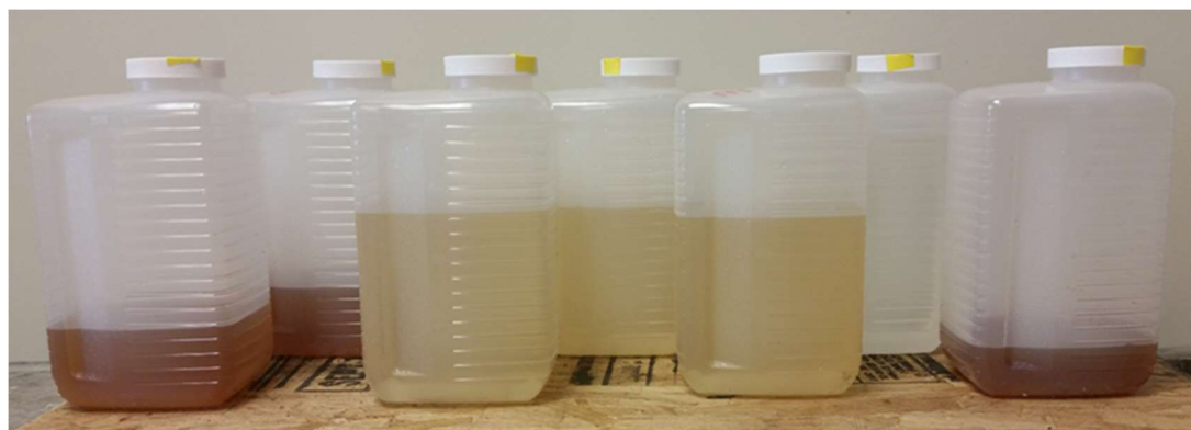
Figure B.2. Green roof runoff collected after Rainfall Event #10.
