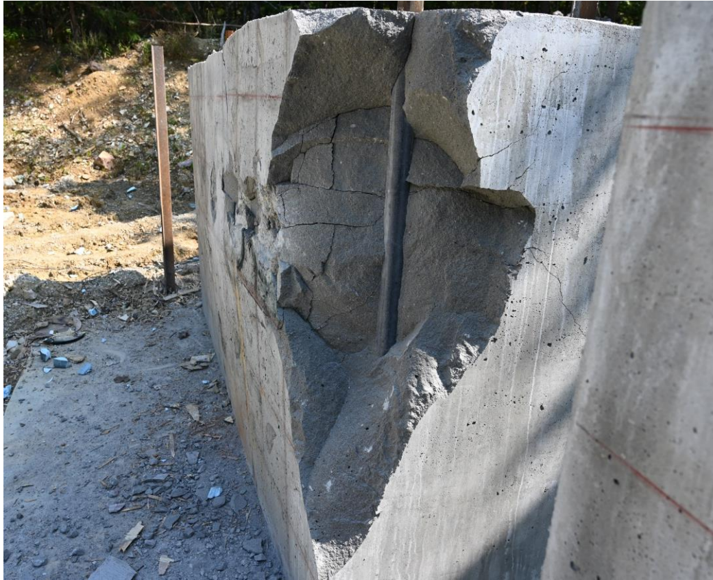
Figure 4.10. 50 psi seal fragmentation planes
