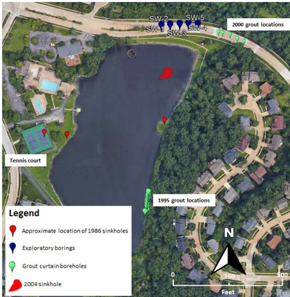
Figure 1.3. Locations of previous sinkholes, exploratory borings and grout injection points.
