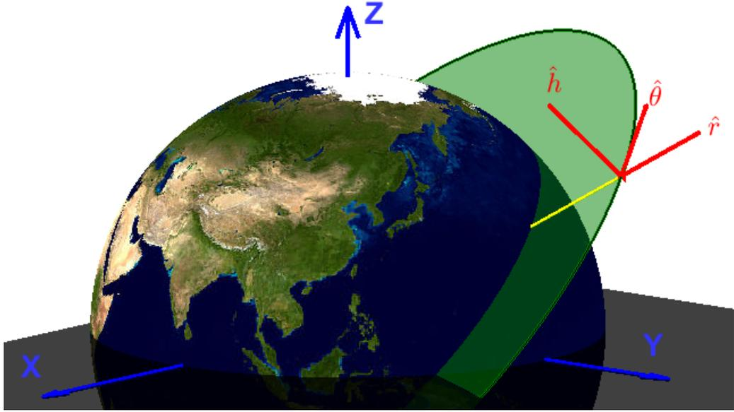
Figure 2.1. Local Vertical Local Horizontal (LVLH) Frame
