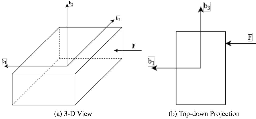
Figure 3.1. Spacecraft Body Frame Example
