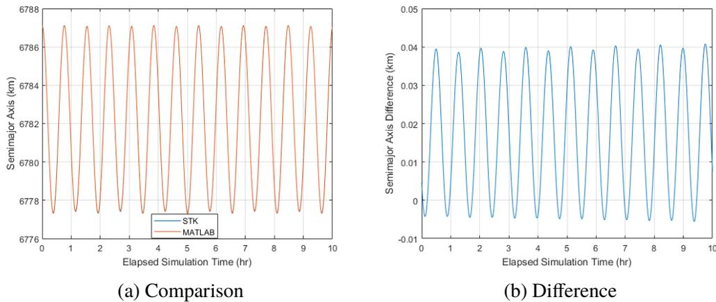
Figure 2. Propagation Comparison and Difference for Semimajor Axis
