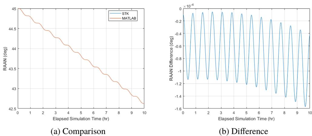
Figure 5. Propagation Comparison and Difference for Right Ascension of Ascending Node
