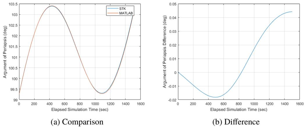
Figure 13. Electric Mode Maneuver Comparison and Difference for Argument of Periapsis
