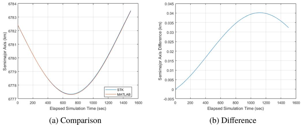
Figure 9. Electric Mode Maneuver Comparison and Difference for Semimajor Axis
