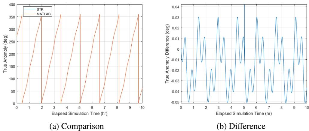
Figure 7. Propagation Comparison and Difference for True Anomaly
