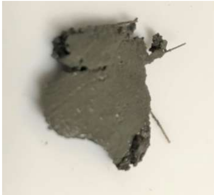
Figure 4.34. Dry Consolidated Mortar Due to High Extrusion Pressure
