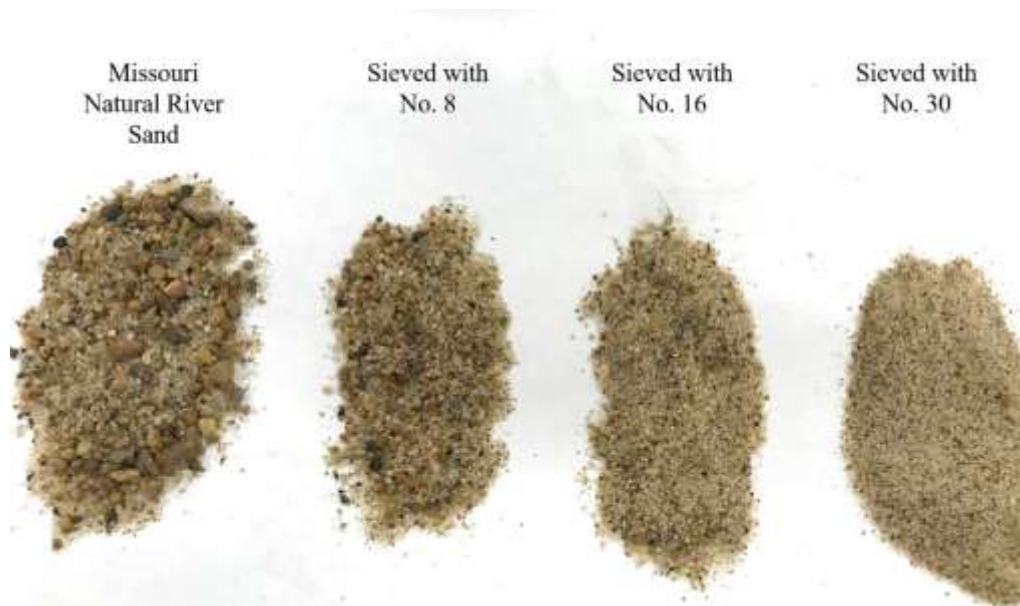
Figure 3.2. Sand Sizes for Blockage Test
