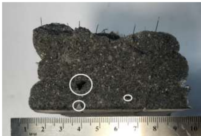
Figure 4.41. Printing Gaps in Cross Section
