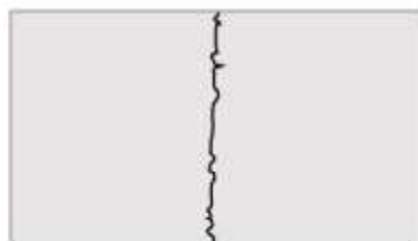
(a) Vertical Crack in Cast Beam
