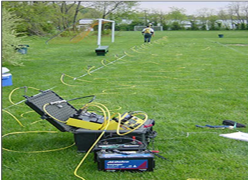
Figure 5.6. The field equipment of the ERT.
