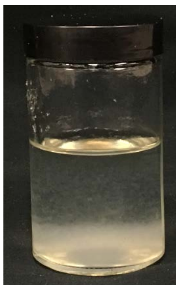
Figure 4.21. Residue of RPPG after degrading by \text{Na}_2\text{S}_2\text{O}_8 (6%) activated by NaOH (12%) (Room temperature)
