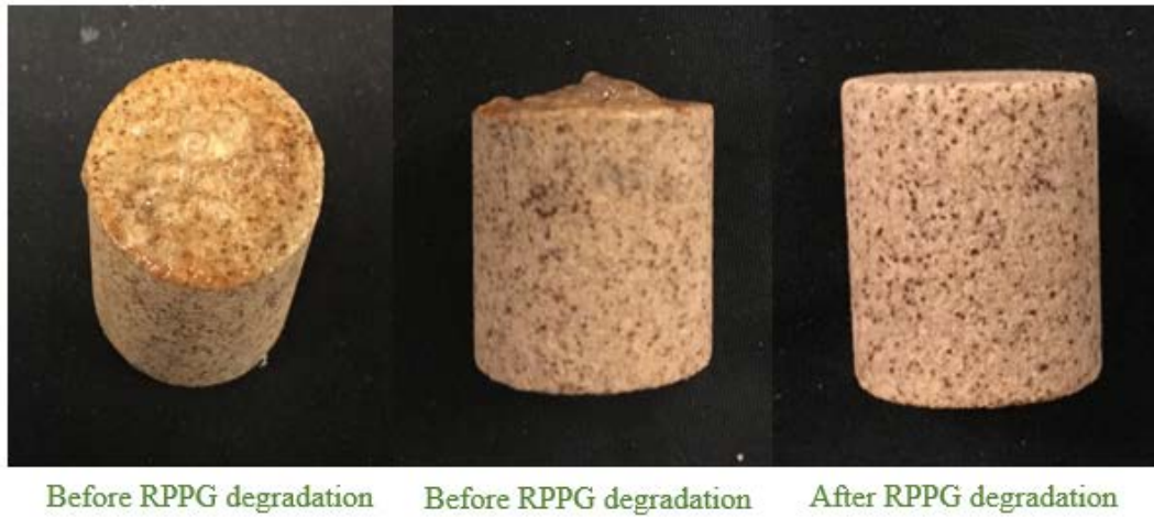
Figure 4.31. Core before RPPG degradation and after RPPG degradation
