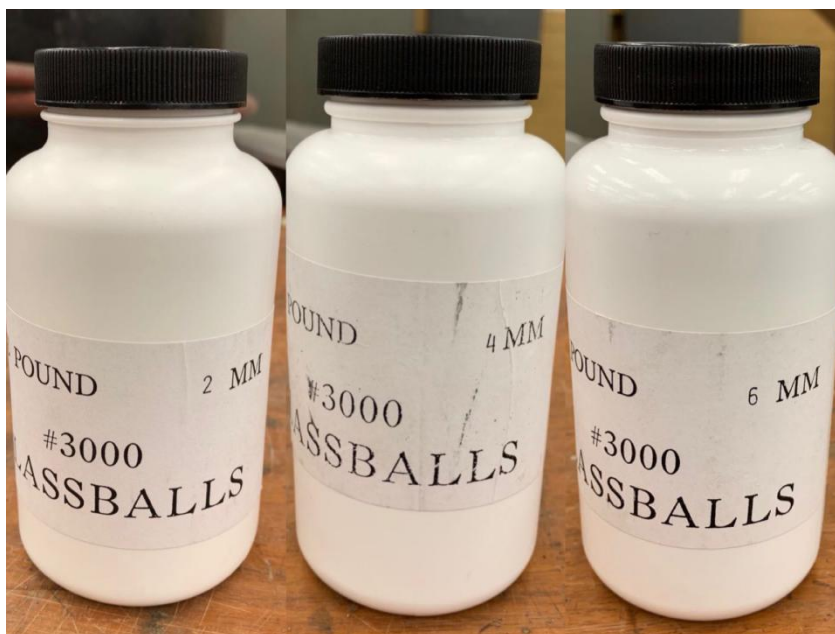
Figure 3.1. Different sizes (2 mm, 4 mm, and 6 mm) of glass beads proppant.
