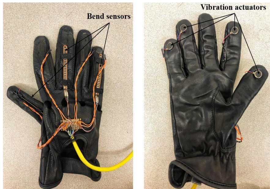
Figure 2.2. (Left) Outer side of the glove with bend sensors on thumb, middle and little fingers. (right) Inner side of the glove with vibration actuators on all except middle finger.
