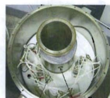
Gamma collimation hole ^3\text{He} tubes (6)
