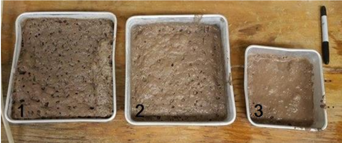
Figure 4.21. A picture of froth products collected at different time ranges when Hy-PAM dispersant was used 1) 0 to 2 min, 2) 2 to 4 min, and 3) 4 to 6 min.
