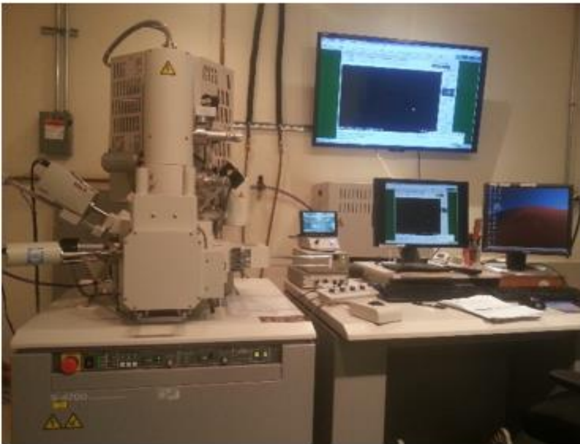
Figure 3.1. Picture of scanning electron microscope used in this study (Hitachi S4700) at Missouri S&T, Rolla, MO.
