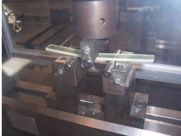
Figure 5.7. Flexure test setup
