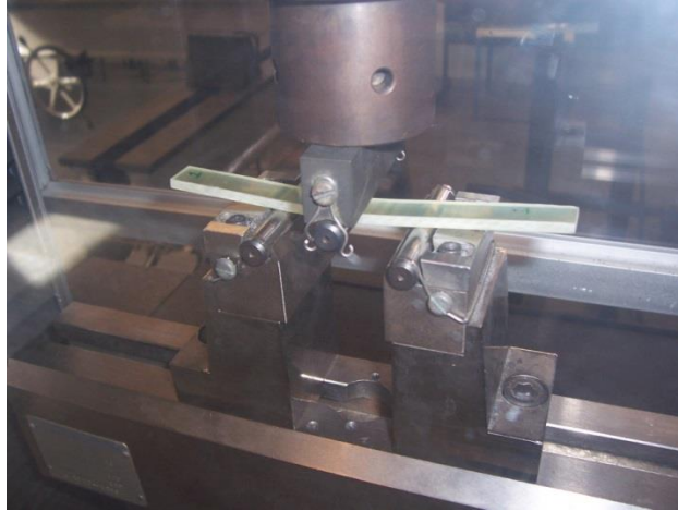
Figure 5.7. Flexure test setup
