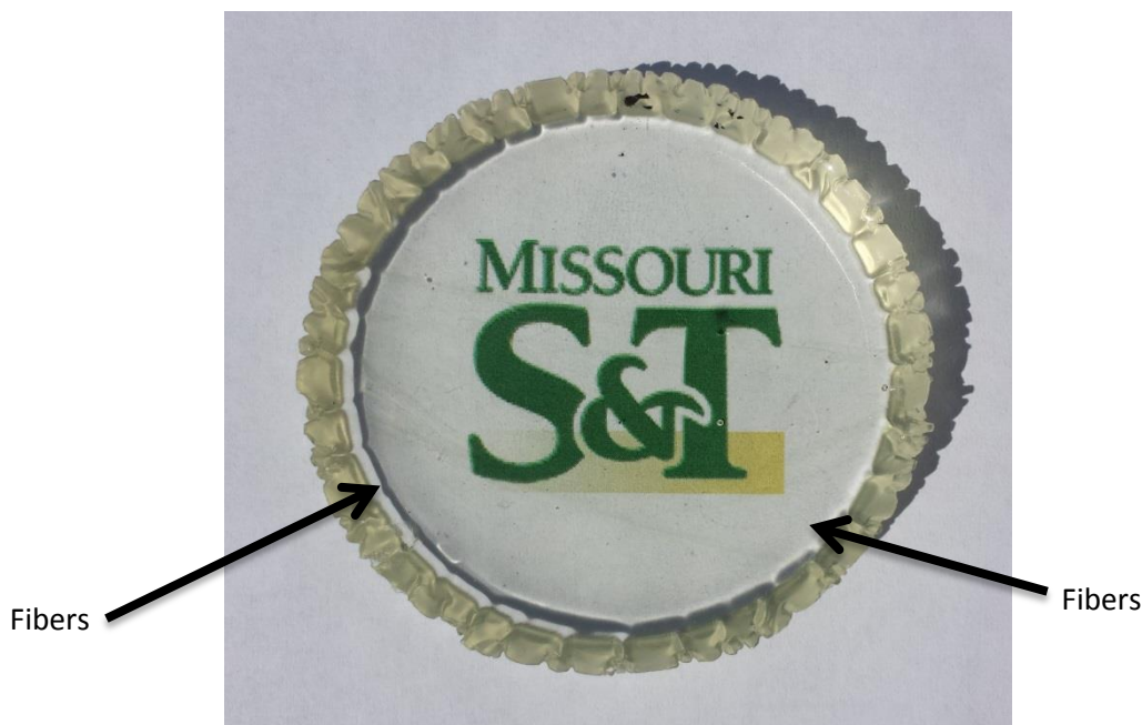
Figure 2.3. Fiber and resin sample for refractive index matching
