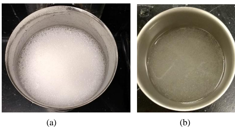
Figure 4.2. Linear gel condition (a) Immediately after mixing (b) After 24 hours of mixing
