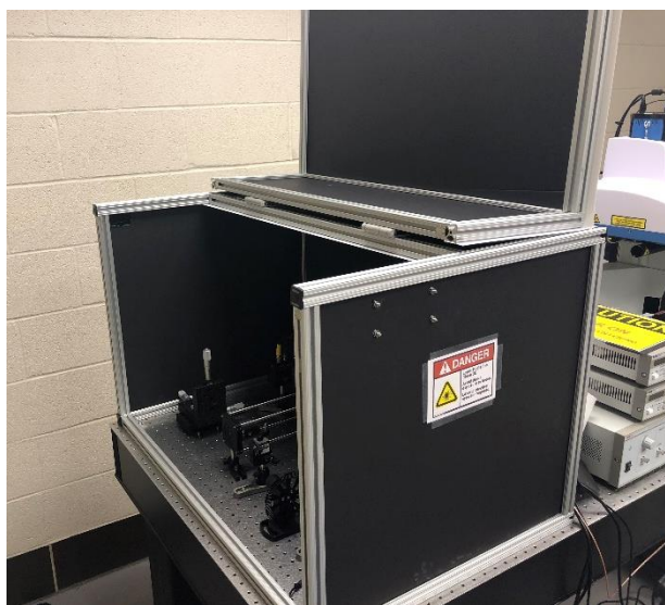
Figure 2.1: Light-proof enclosure for optical components.
