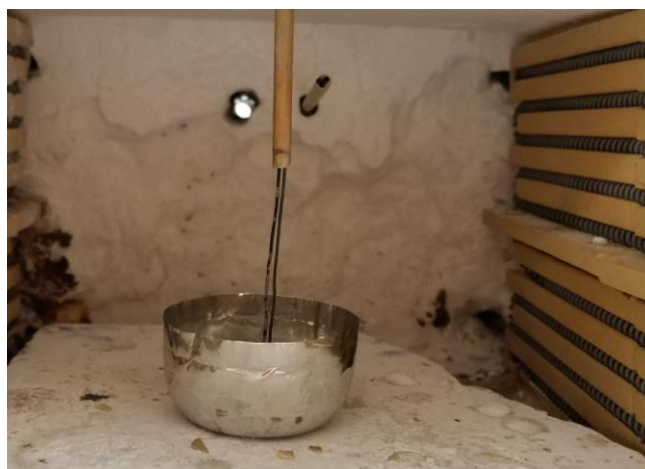
Figure 5. Furnace cool experiment with embedded thermocouple.
