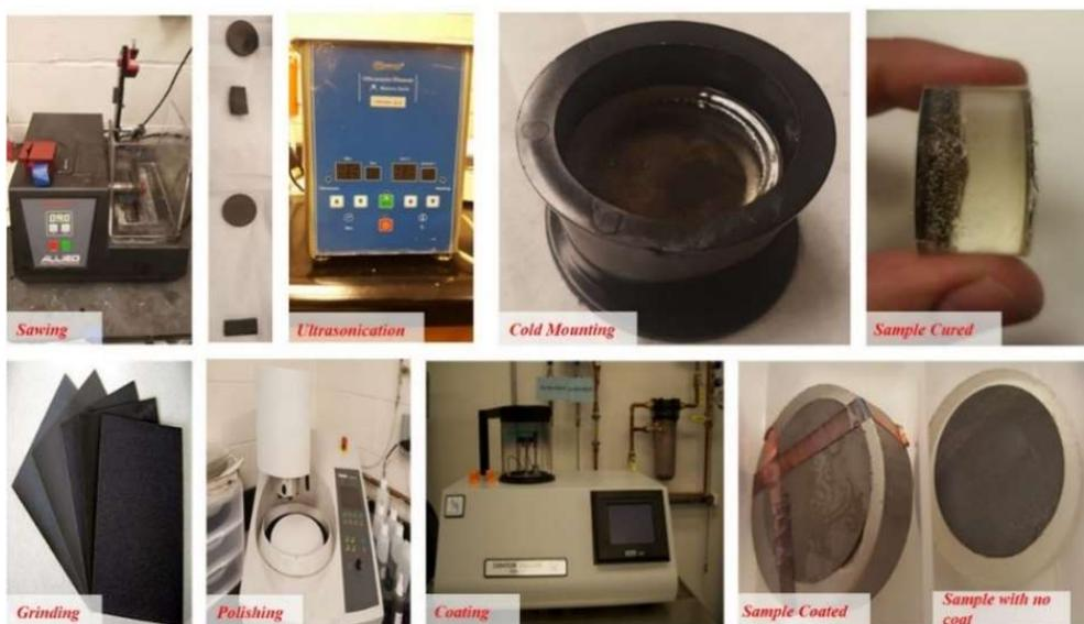
Figure 3.6. SEM samples preparation.
