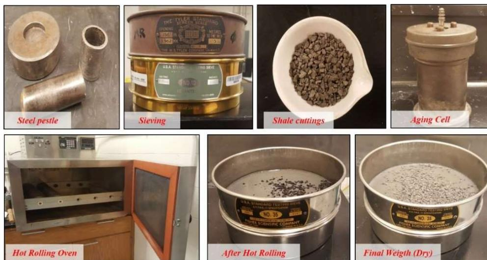
Figure 3.31. Cutting dispersion test.
