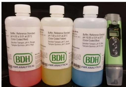
Figure 3.26. pH meter and buffer solutions. Missouri S&T.
