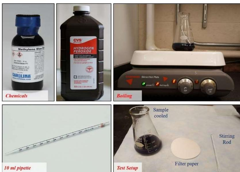
Figure 3.9. Materials and steps for CEC procedure.
