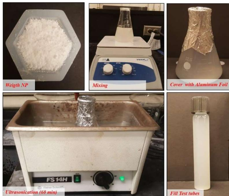
Figure 3.15. Sample preparation for aqueous stability test.
