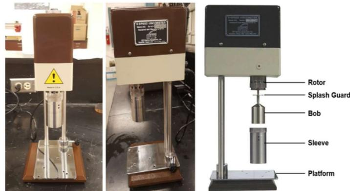
Figure 3.27. 8-speed OFITE viscometer. Missouri S&T.
