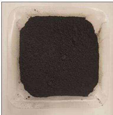
Figure 3.20. Conventional LCM graphite.
