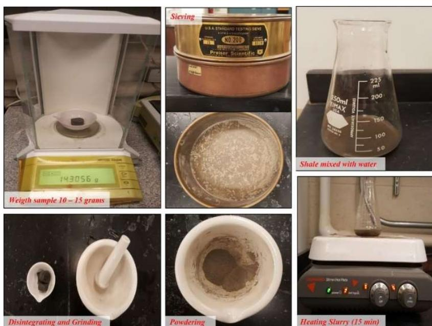
Figure 3.8. CEC shale slurry preparation.
