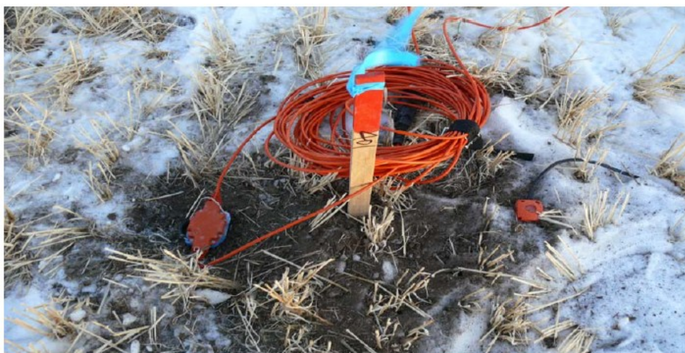
Figure 1.10. Right SM7 geophone, left DSU3 MEMS sensor at one station (Bertram et al., 2008).
