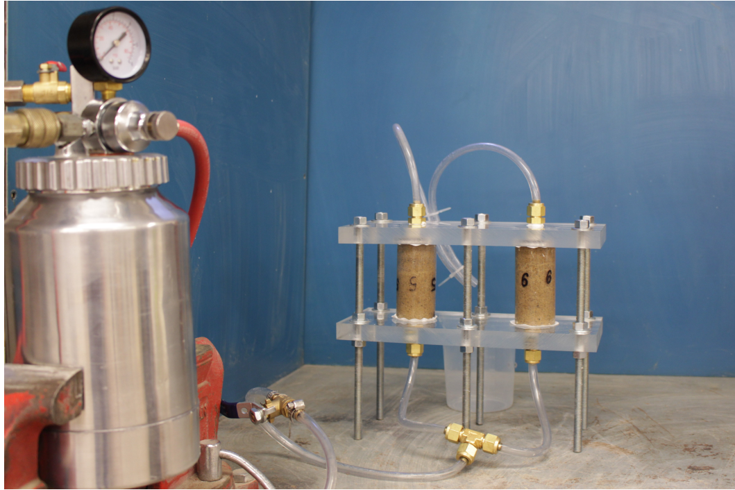
Figure 2.11. Injection of Sand Columns.
