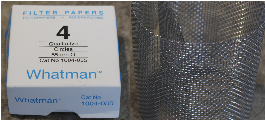
Figure 2.9. Filter Paper (left) and Steel Mesh (right).
