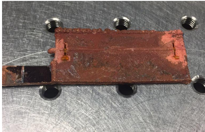
Figure 4.1. The photo of copper slide with embedded optical fiber sensor
