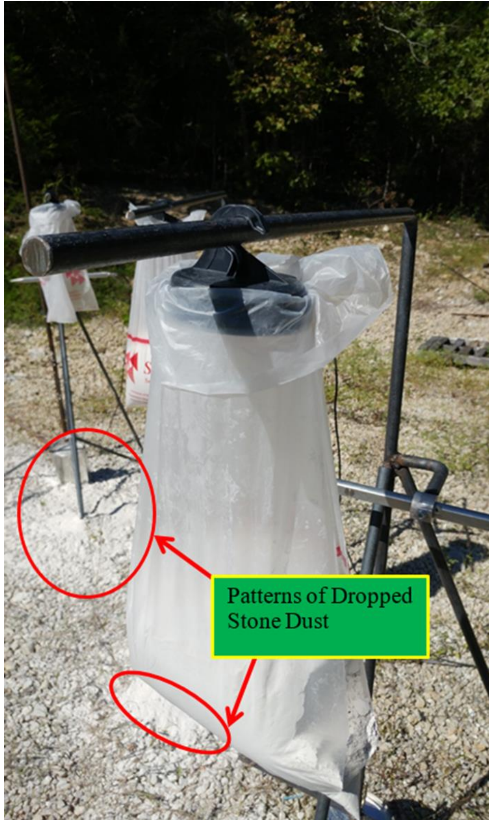
Figure 3.5: Picture Showing Typical Pattern of Dropped Stone Dust
