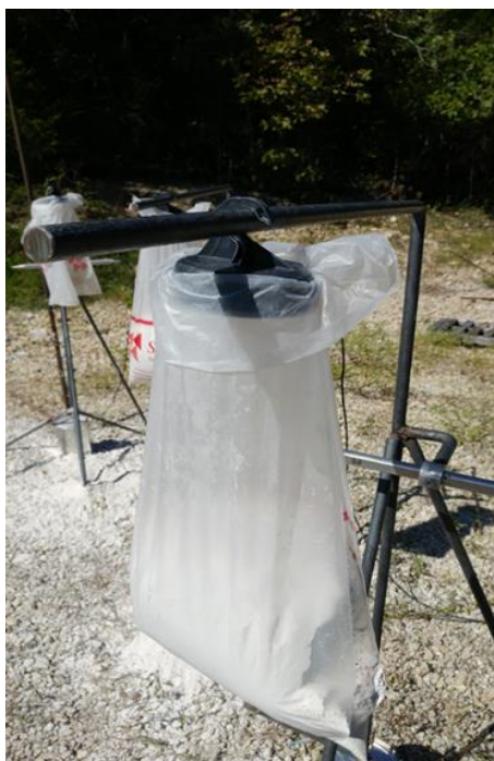
Figure C1.2: 120g C4 Test Bag Position 3 (9 ft)
