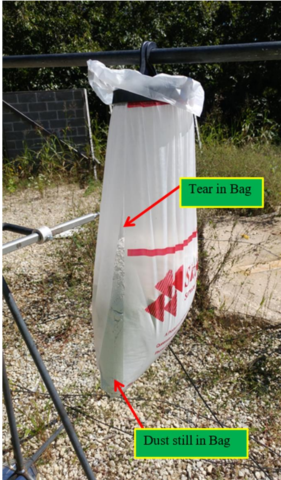
Figure 3.6: Picture Showing Split in Bag Typical at Greater Distances
