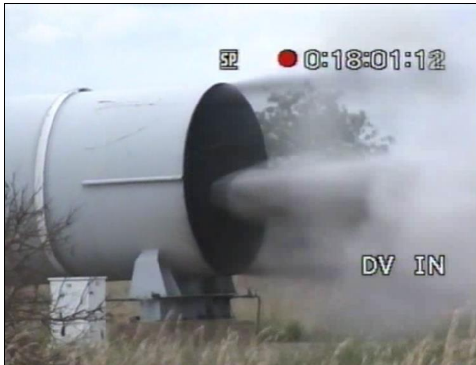
Figure 2.4: Bag Explosion Testing at Kloppersbos Testing Facility
