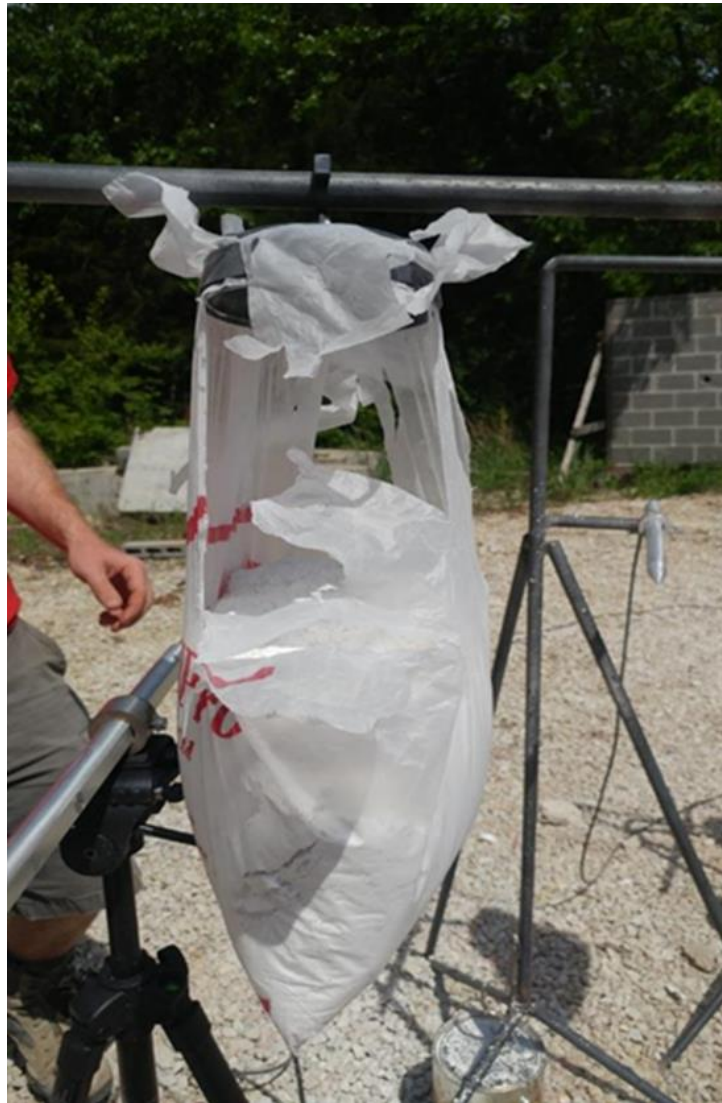
Figure C1: 60g C4 Test Bag Position 1 (5 ft)
