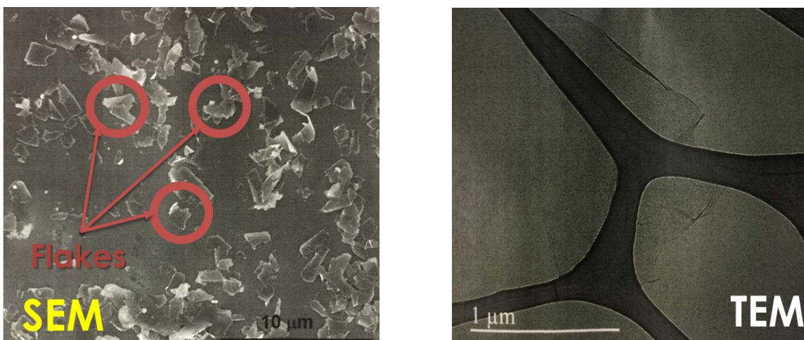
Figure 1. Shows SEM & TEM of GNPs (Provided by Nanographene Inc.).
