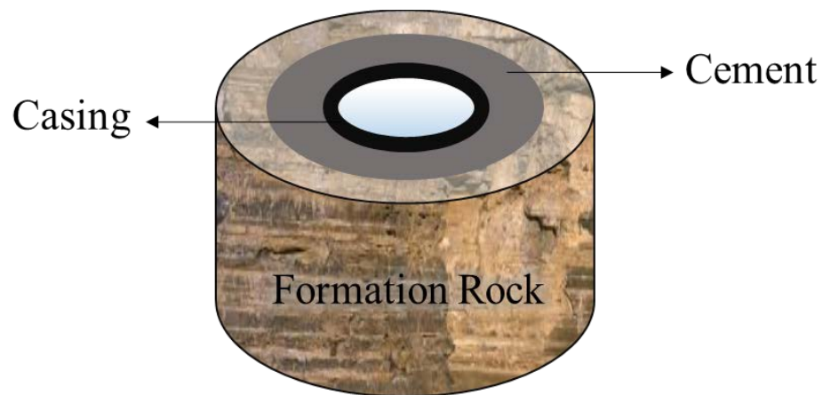
Figure 1. A cross-section of a wellbore showing the role of the cement between the casing and the formation.
