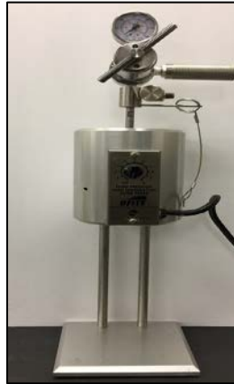
Figure 5.7. A filtrate press test equipment.
