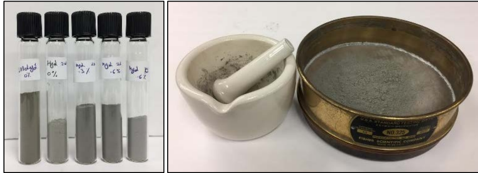
Figure 5.2. Samples of cement and the sieve (325 mesh).
