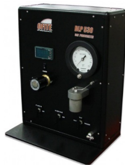
Figure 5.16. Example of Helium Porosimeter (OFI Testing Equipment).
