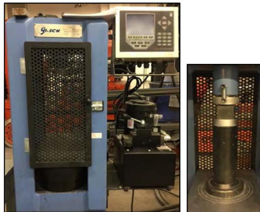
Figure 5.11. An example of hydraulic press testing machine.
