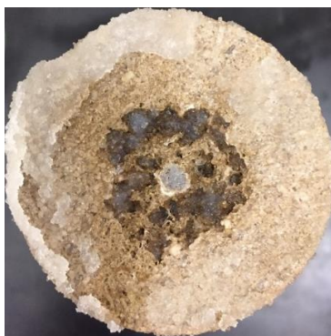
Figure 4.7. The image of the acid diversion coverage (20 min after injecting acid)
