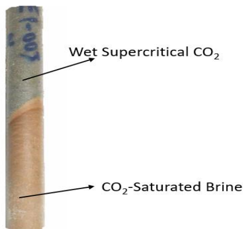
Figure 3.5. The cement exposed to different phases of CO 2 (Bu et al., 2010)
