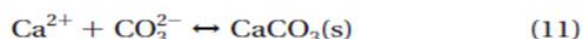
Figure 3.27. Equations of microbial (or biofilm) induced carbonate precipitation (Andrew C. Mitchell et al., 2010)
