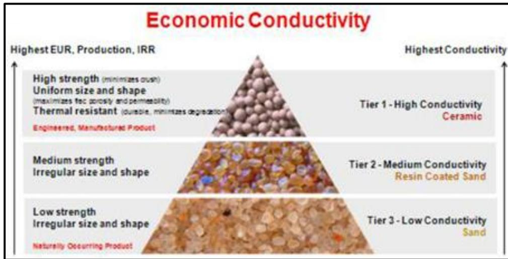
Figure 1.7. Proppant conductivity pyramid showing three tiers of proppant.( Gallagher et al. 2011)
