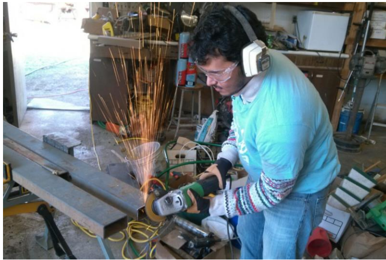
Figure 4.1: The process of constructing the actuator frame. Eliminating the sharp edges of the actuator frame to make it hand safe.
