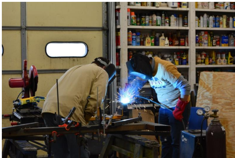
Figure 4.2: The welding process of the actuator frame.
