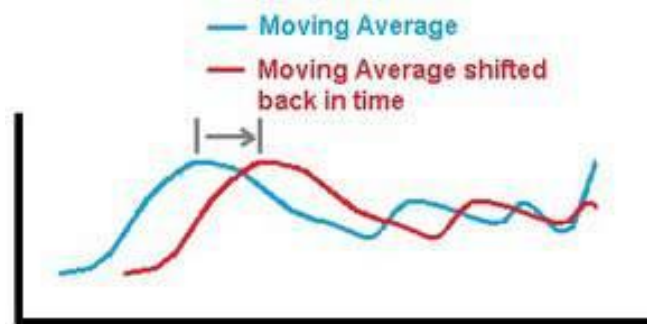
Figure 5.5: Backward moving average. The backward moving average means that data cannot be used to predict the future events.
