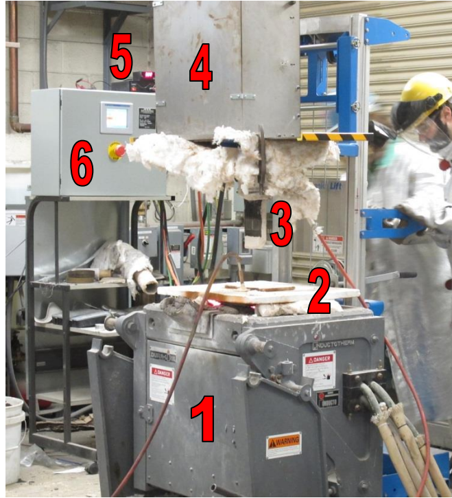
Figure 2.1. Dip tester setup. 1: 200 lb induction furnace, 2: furnace lid, 3: dipping paddle with textured copper blocks, 4: servo motor enclosure, 5: melt-sensing circuit's power supply and voltmeter, and 6: dip tester electronics enclosure.
