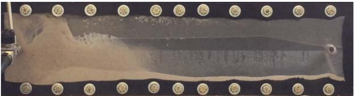
Figure 4.59. Small Proppant Floated High up to the Upper Bound of the Slot, While Most of Large Proppant Settled Rapidly
