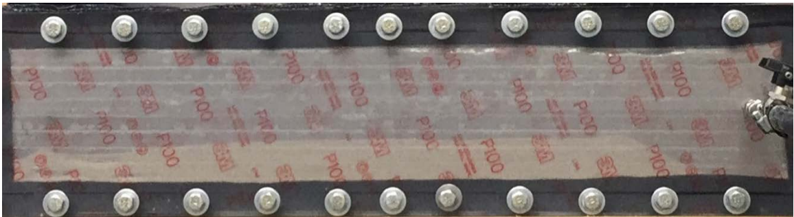
Figure 4.8. Low Roughness Fracture Slot
