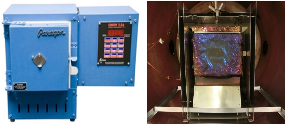
Figure 3.3. Furnace. (Left: Original kiln model. Right: Repurposed kiln sitting in outer box of insulation).
