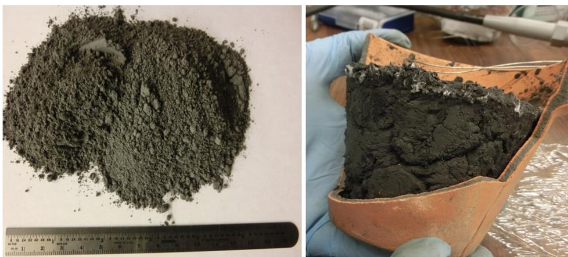
Figure 3.15. Orgueil Simulant. A) Granular form. B) Consolidated form while being removed from clay mold.
