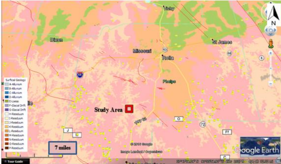
Figure 2.6. Geological map of study area (Courtesy of Google Earth). The study area is marked as red square. Mapped faults and lineaments (marked as blue lines) nearby the study area is trending mostly southeast-northwest. Yellow dots show locations of known sinkholes.
