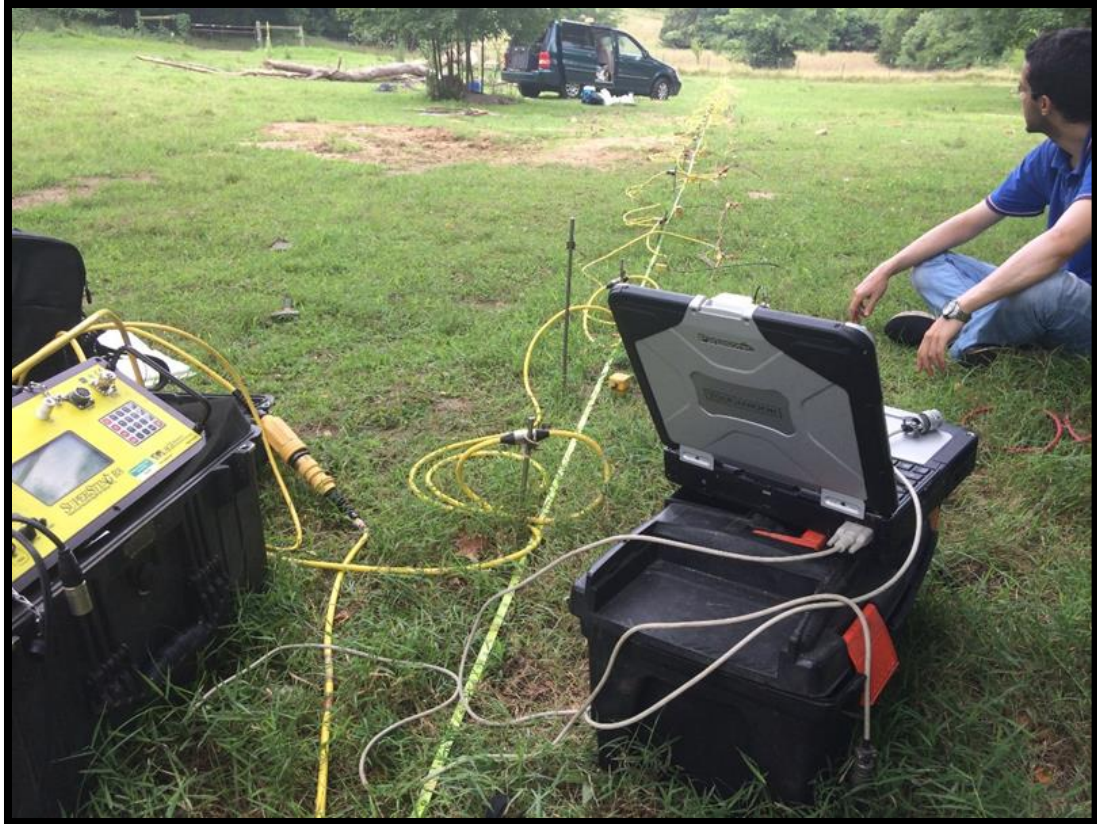
Figure 5.2. Showing the acquisition of ERT data.
