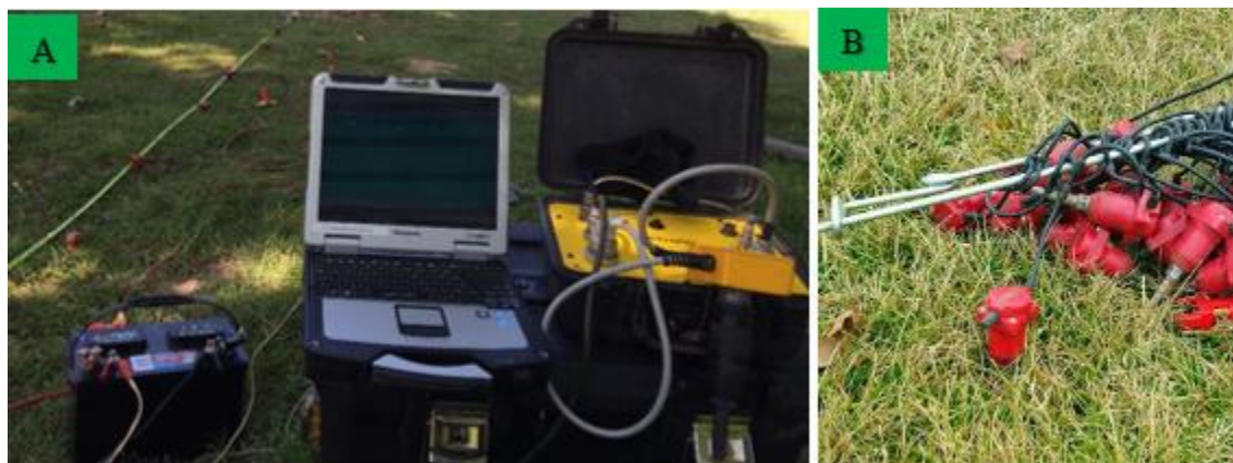
Figure 5.5. MASW field setup, a) seismograph, laptop and 12V battery and b) 4.5 Hz Geophones with spikes.
