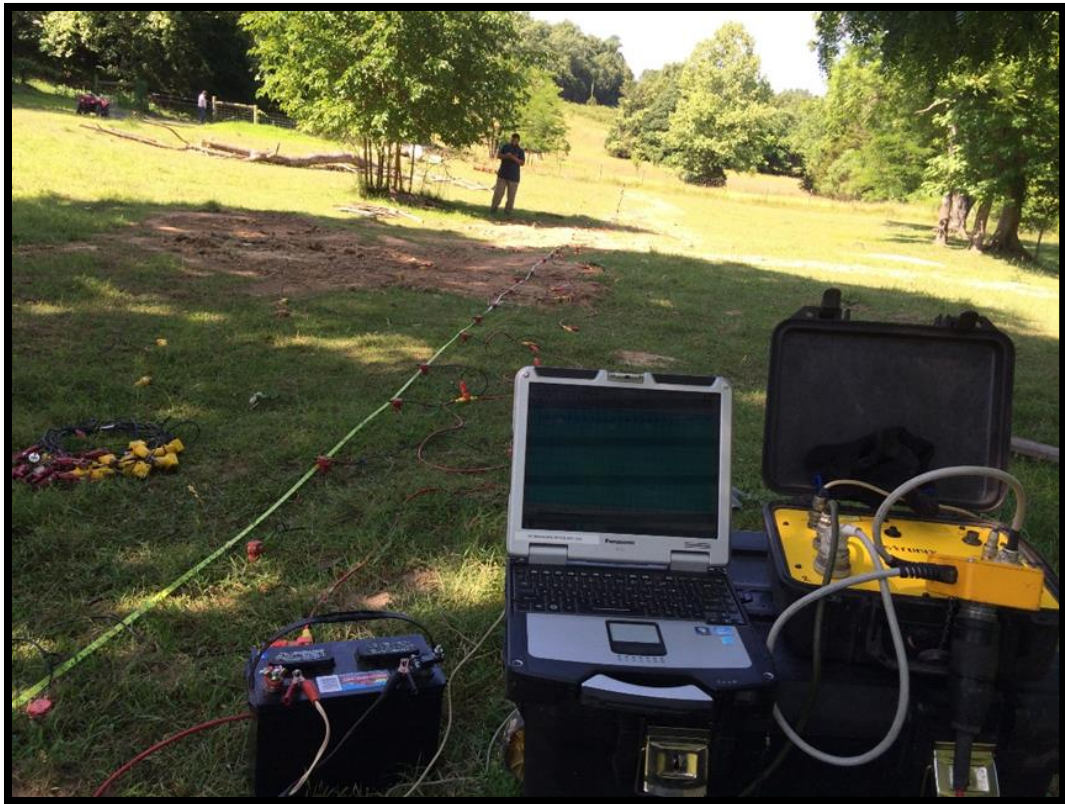
Figure 5.1. Showing the acquisition of MASW data.
