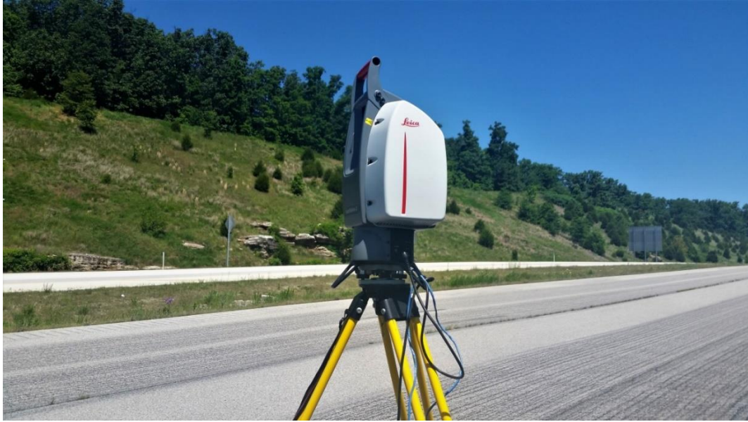
Figure 2.11. Leica Scanstation 2 Post-setup
