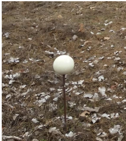
Figure 2.6. Typical Control Rod With 6" (152.4 mm) Target Embedded outside the Slide Boundaries
