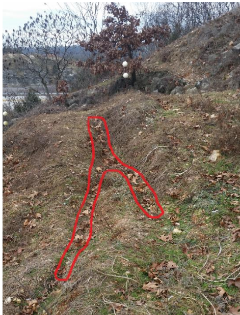
Figure 3.9. Divot on Upper Middle Portion of the Slide (Divot Boundaries Outlined in Red)
