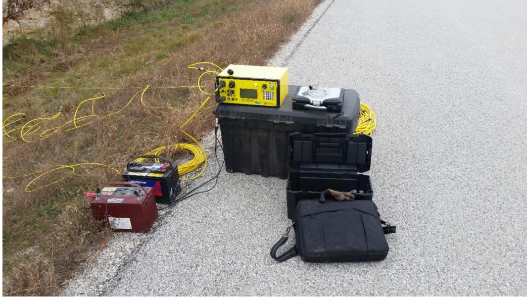
Figure 2.26. AGI SuperSting R8 Multichannel Electrode System
