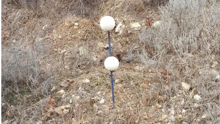
Figure 2.7. Typical Floating Target Rod with Twin 4" (101.6 mm) Targets Embedded within Slide Boundaries
