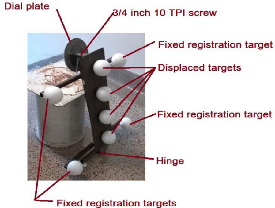
Figure 2.53. Displacement Rig (Maerz et al., 2016)
