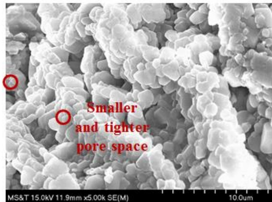
Fig 4.11.SEM results for 40K Series gel swollen in 0.25% NaCl solution after exposure to CO<sub>2</sub> at 10 µm
