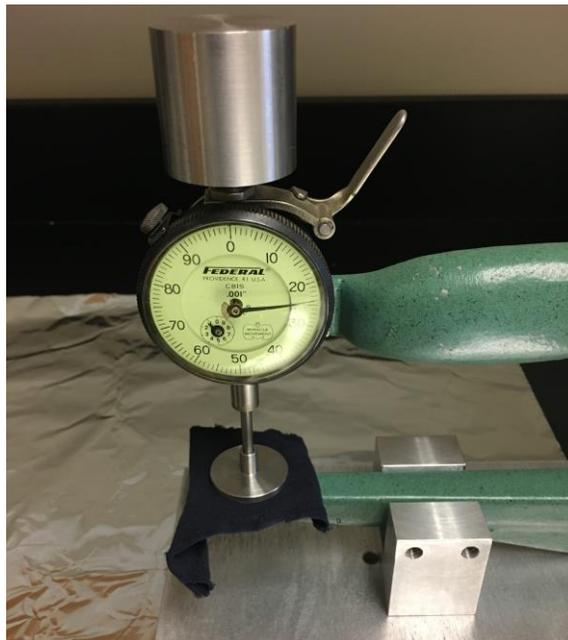
Figure 3.2: Fabric Thickness Gauge
