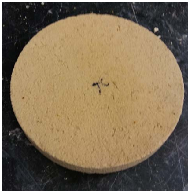
Figure 3.9: Finished filter disk
