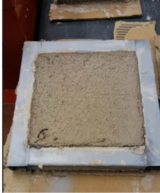
Figure 3.7: Pressed filter block before firing
