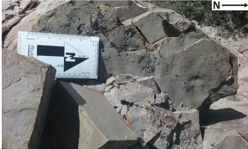
Figure D.6. Ripple marks on block of upright Triassic Virgin Limestone Member (TRmv). The crests show this is the upper surface of the bedding plane, which dips east (upright). However, the heavily disturbed nature of the top of the ridge suggests this piece may not be representative (not in place).
