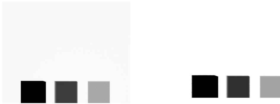
(a) MCNP radiography image of lead, aluminum, and water with a detector resolution of 578 \times 726 (b) ADVANTG radiography image of lead, aluminum, and water with a detector resolution of 578 \times 726
