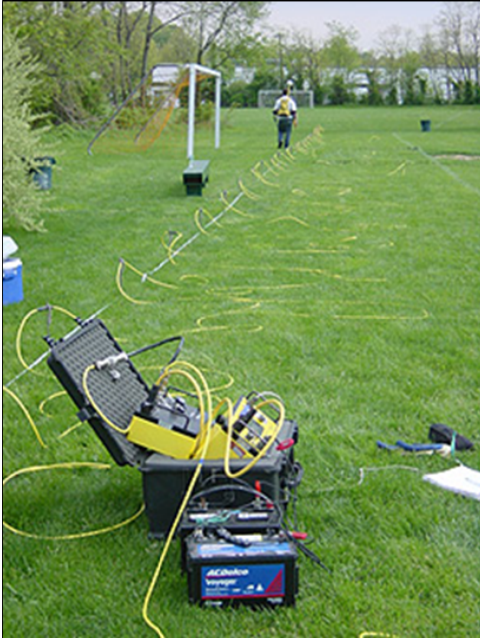
Figure 7.1 Supersting resistivity unit that used in ERT data acquisition. (Source: https://www.indiamart.com/proddetail/electrical-resistivity-survey-service-6174260997.html ).
