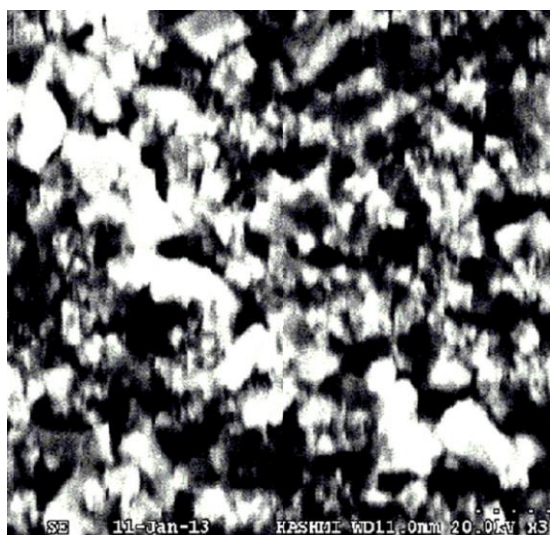
Figure 2.2 SEM photomicrographs of natural magnesite ore (Raza and Zafar 2013)
