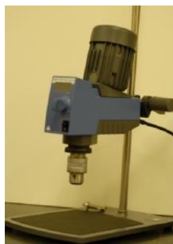
Figure 3.7. (a) Mechanical stirrer; (b) disposable plastic pipette of 23 mL in volume
