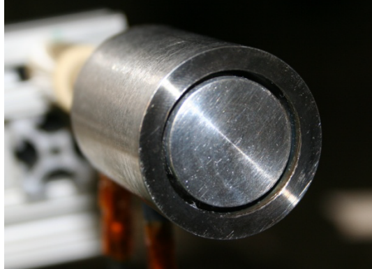
Figure 2.2: Faraday Probe integrated into large vacuum chamber diagnostic probe arm.
