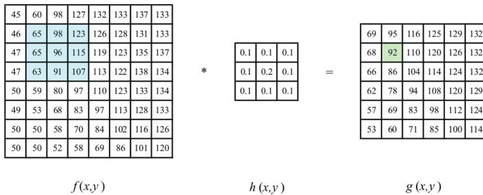
Figure 5.1. Two dimensional image filtering process [13]
