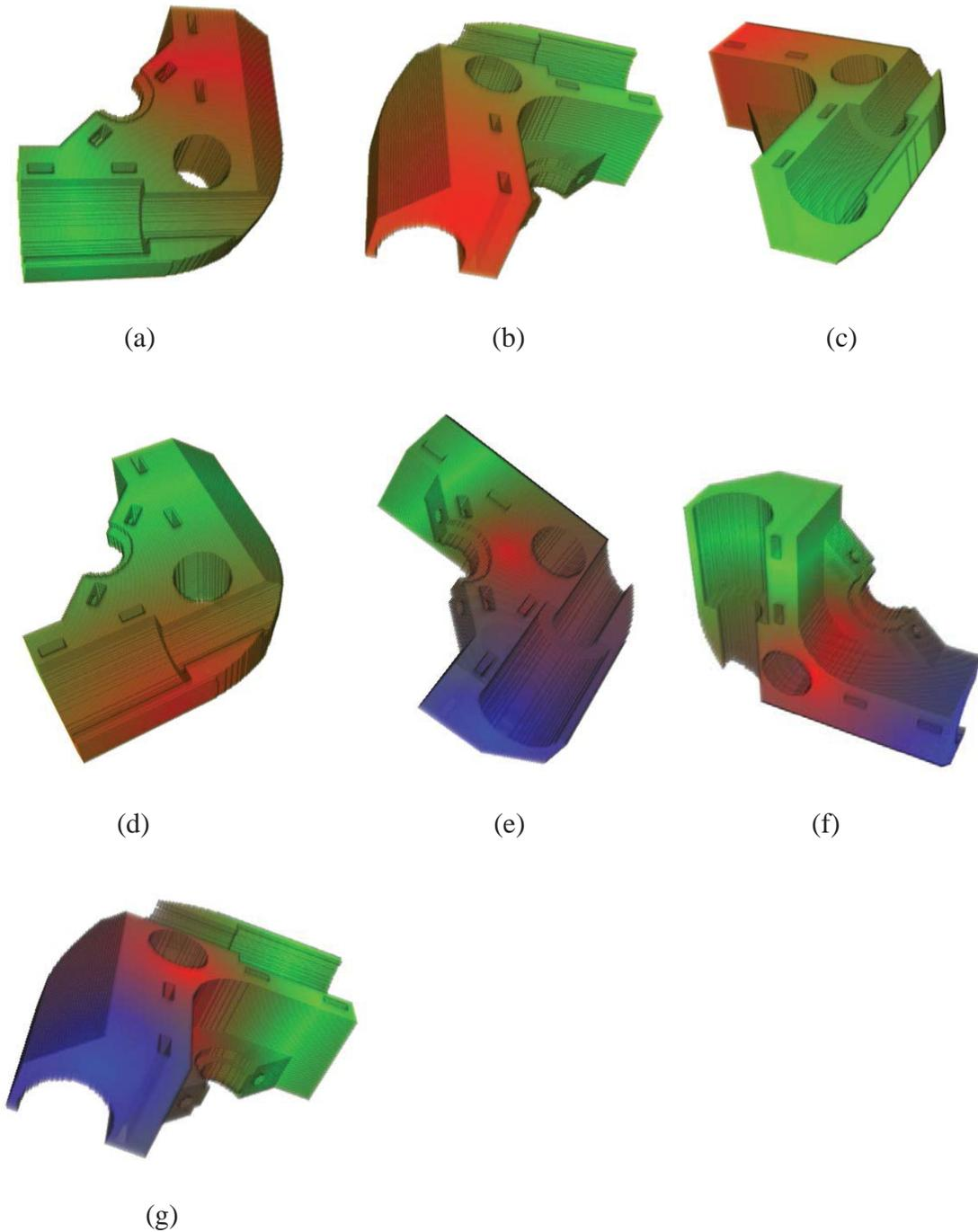
Figure 4.5. FGMs modeling using different control sources in drucken (a) two planar control sources (b) (c) Two point control sources. (d) Two different types of control sources: one planar and one point control source. (e) (f) (g) Three different types of control sources: one planar, one point and one line control source.
