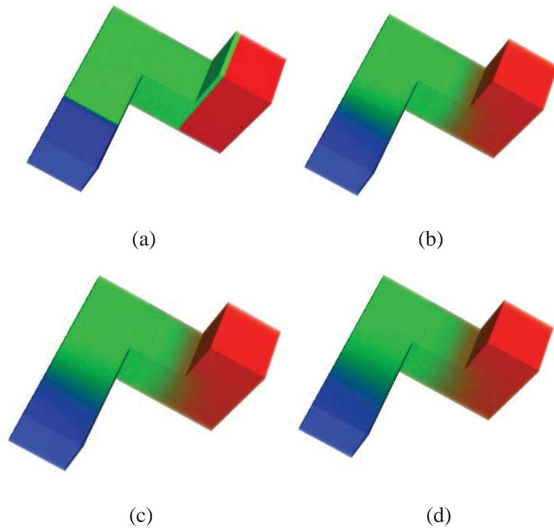
Figure 5.7. (a) Original default model, voxel resolution at  $100 \times 100 \times 68$  (b) Average filtering with kernel size = 5 (c) Average filtering with kernel size = 15 (d) Average filtering with kernel size = 25
