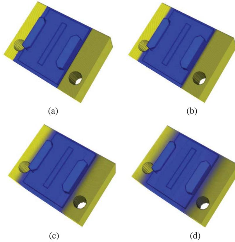
Figure 5.8. (a) Original default model, voxel resolution at  $100 \times 175 \times 135$  (b) Average filtering with kernel size = 5 (c) Average filtering with kernel size = 15 (d) Average filtering with kernel size = 25
