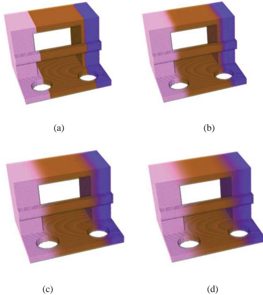
Figure 5.5. (a) Original default material reference feature defined, voxel resolution at  $100 \times 144 \times 122$  (b) Gaussian filtering with  $\sigma = 5$  and kernel size = 11 (c) Gaussian filtering with  $\sigma = 5$  and kernel size = 21 (d) Gaussian filtering with  $\sigma = 11$  and kernel size = 21
