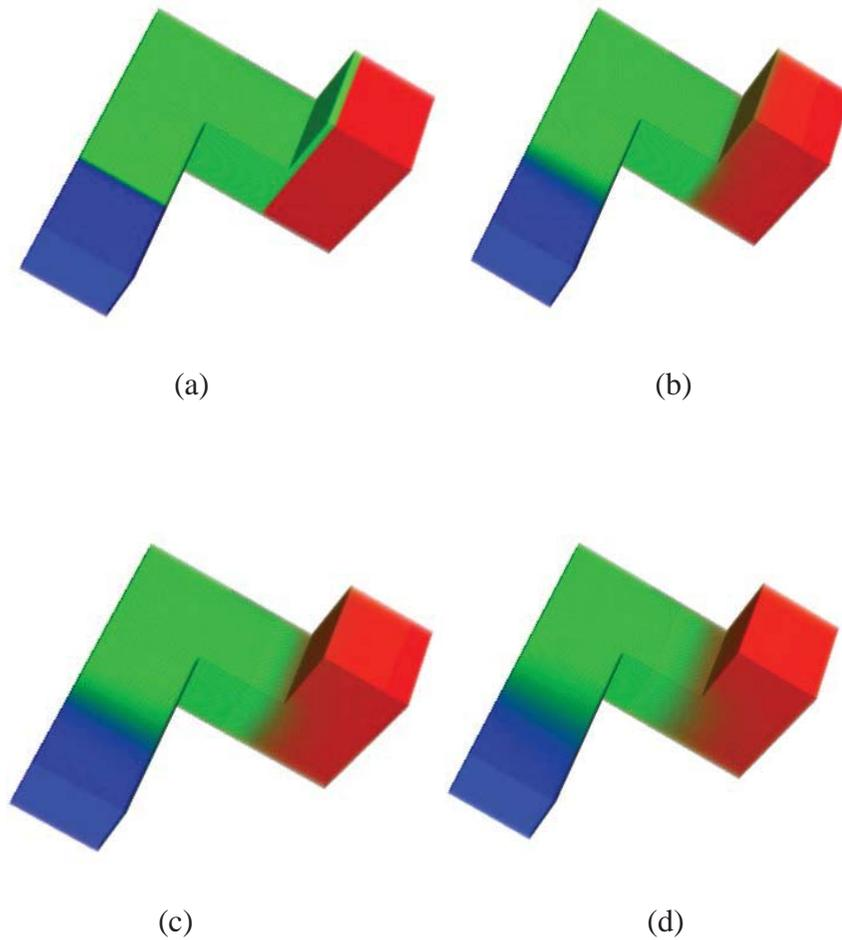
Figure 5.4. (a) Original default material reference feature defined, voxel resolution at  $100 \times 100 \times 68$  (b) Gaussian filtering with  $\sigma = 5$  and kernel size = 15 (c) Gaussian filtering with  $\sigma = 5$  and kernel size = 25 (d) Gaussian filtering with  $\sigma = 15$  and kernel size = 25
