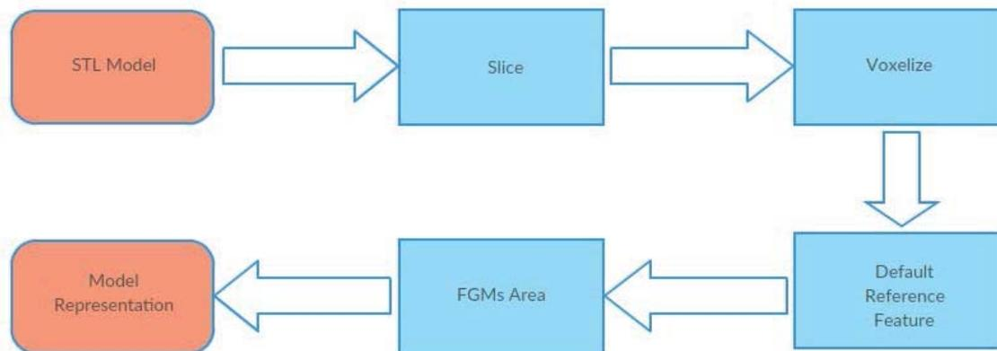
Figure 3.1. FGMs modeling design pattern
