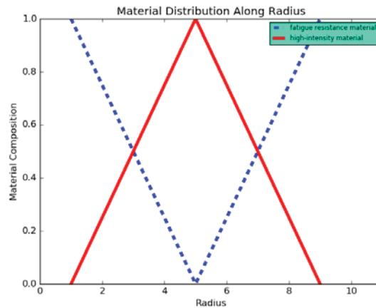
Figure 7.2. Material composition distribution along radius in ring
