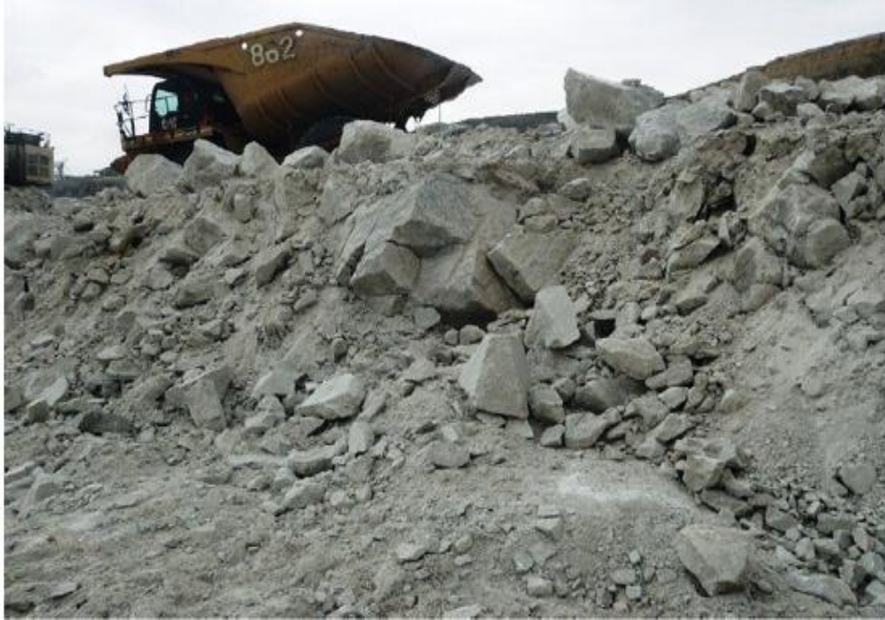
Figure 1.1. Rock formation stationary after blasting
