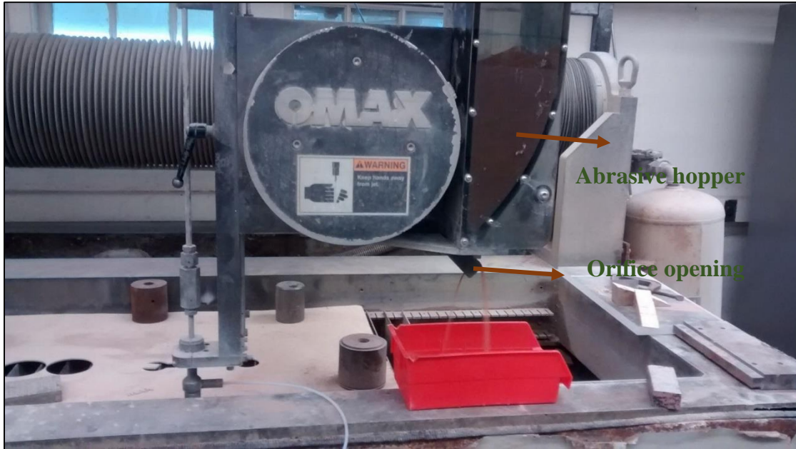
Figure 4.9. OMAX waterjet systems gravity controlled abrasive feeder
