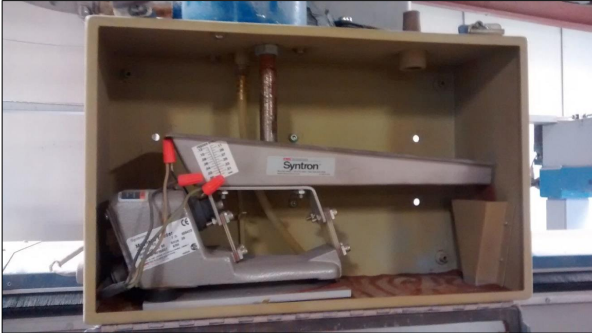
Figure 4.2. Syntron vibratory electromagnetic abrasive feeder in PaR systems
