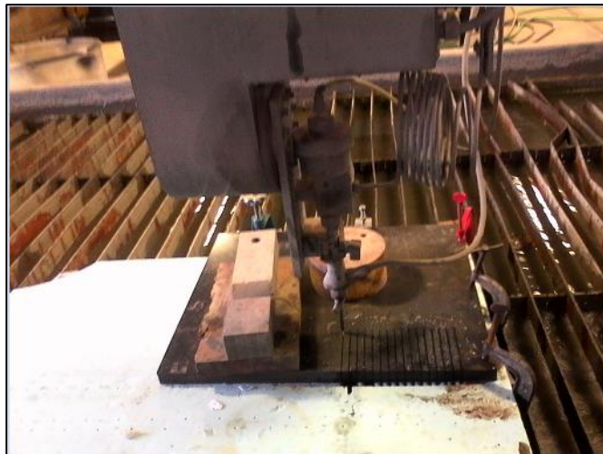
Figure 6.6. AWJ cutting of stack of four \frac{1}{4} " thick composites
