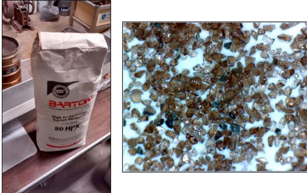
Figure 4.4. 80 HPX® Barton garnet used for the experiment (Batch number HR 060180) and Microscope observation (60X)
