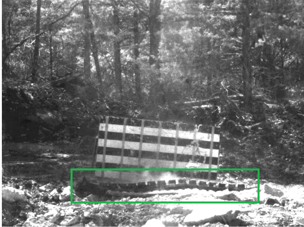
Figure 6.1 Blasting Mat Centered Over Borehole
