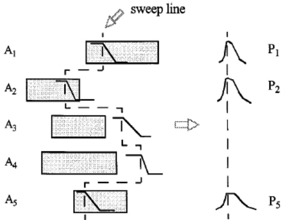
Figure 2.2 Timing Window Versus Aggressor Alignment [4]
