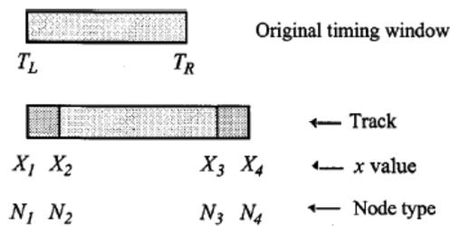
Figure 2.5 Timing Window Adjustment (Stretched and Expanded)
