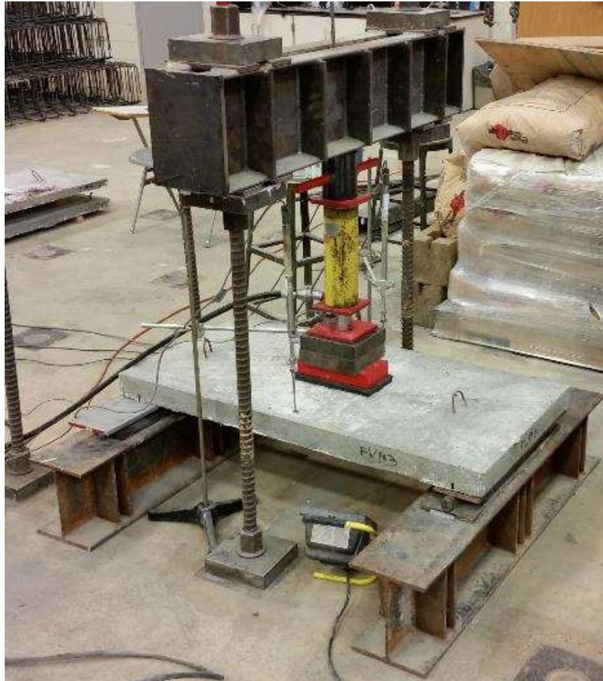
Figure 6.19. Panel FUN3 test setup
