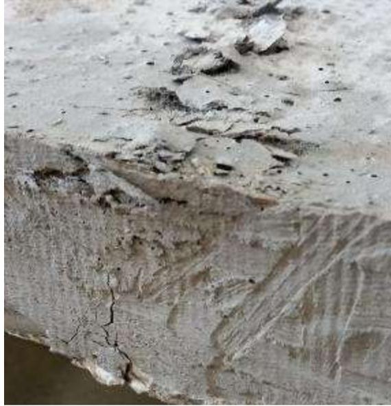
Figure 6.49. Tensile crack on panel SUC2
