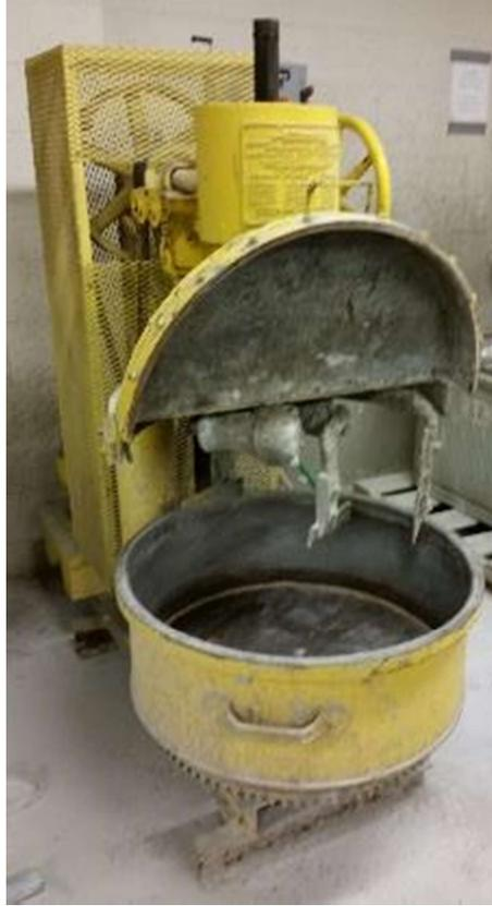
Figure 5.8. High-shear mixer
