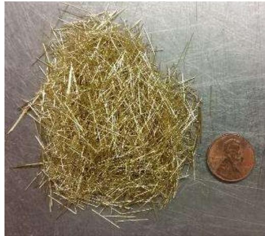
Figure 4.6. Steel fibers
