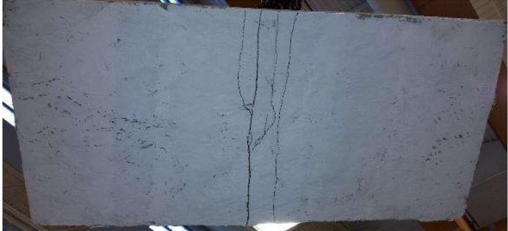
Figure 6.27. Crack pattern formation at the tension face of panel FUN2
