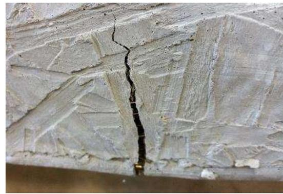
Figure 6.14. Tensile crack on panel FUW3
