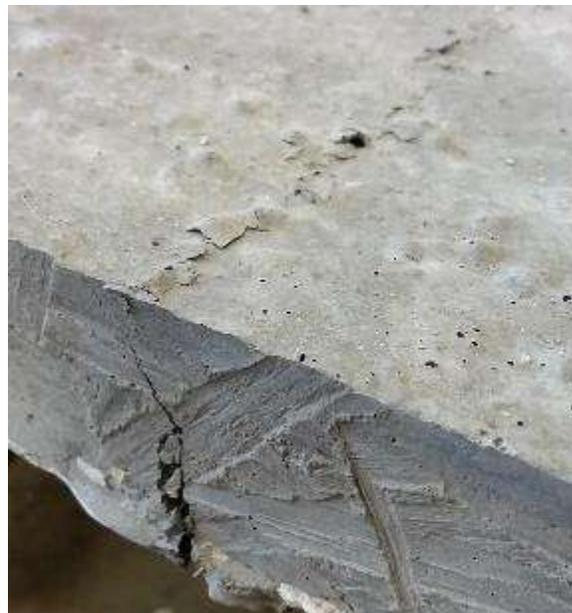
Figure 6.55. Tensile crack on panel SUN2
