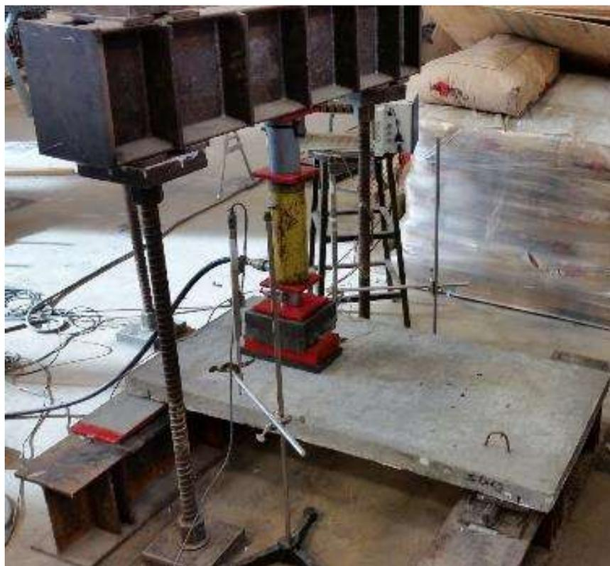
Figure 6.48. Panel SUC2 test setup
