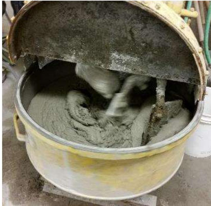
Figure 5.9. UHPC batching
