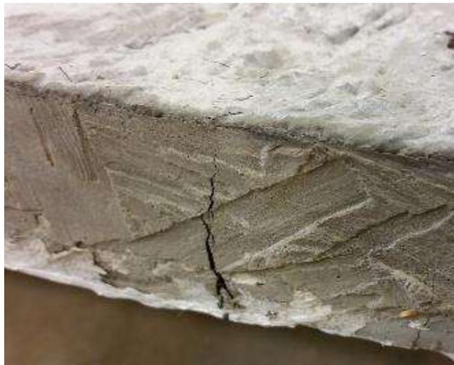
Figure 6.26. Tensile crack on panel FUN2
