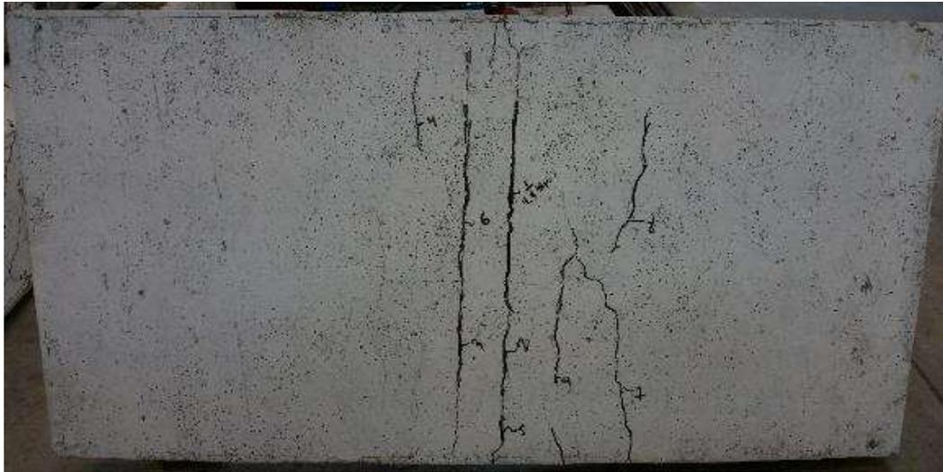
Figure 6.2. Crack pattern formation at the tension face of panel FCC3
