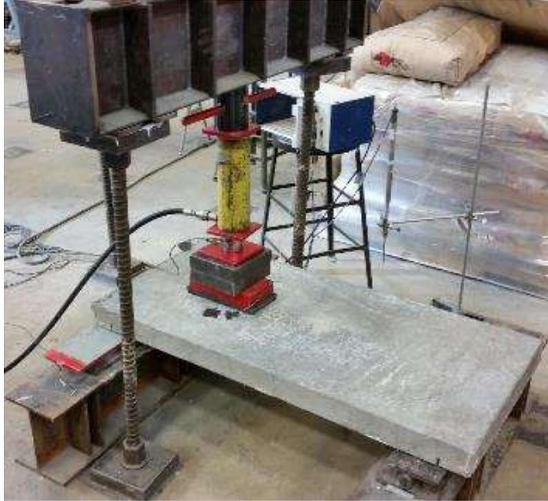
Figure 6.43. Panel SUN3 test setup
