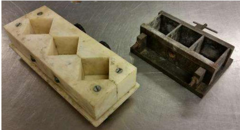
Figure 5.3. Molds for 2-in. (50 mm) cubes
