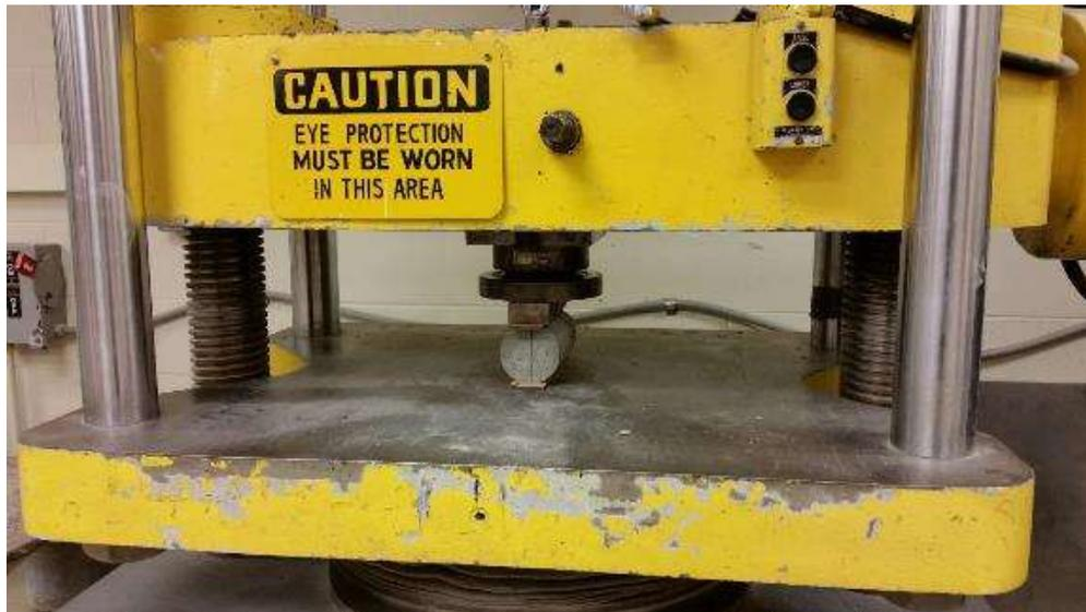
Figure 5.5. Split tensile strength test setup
