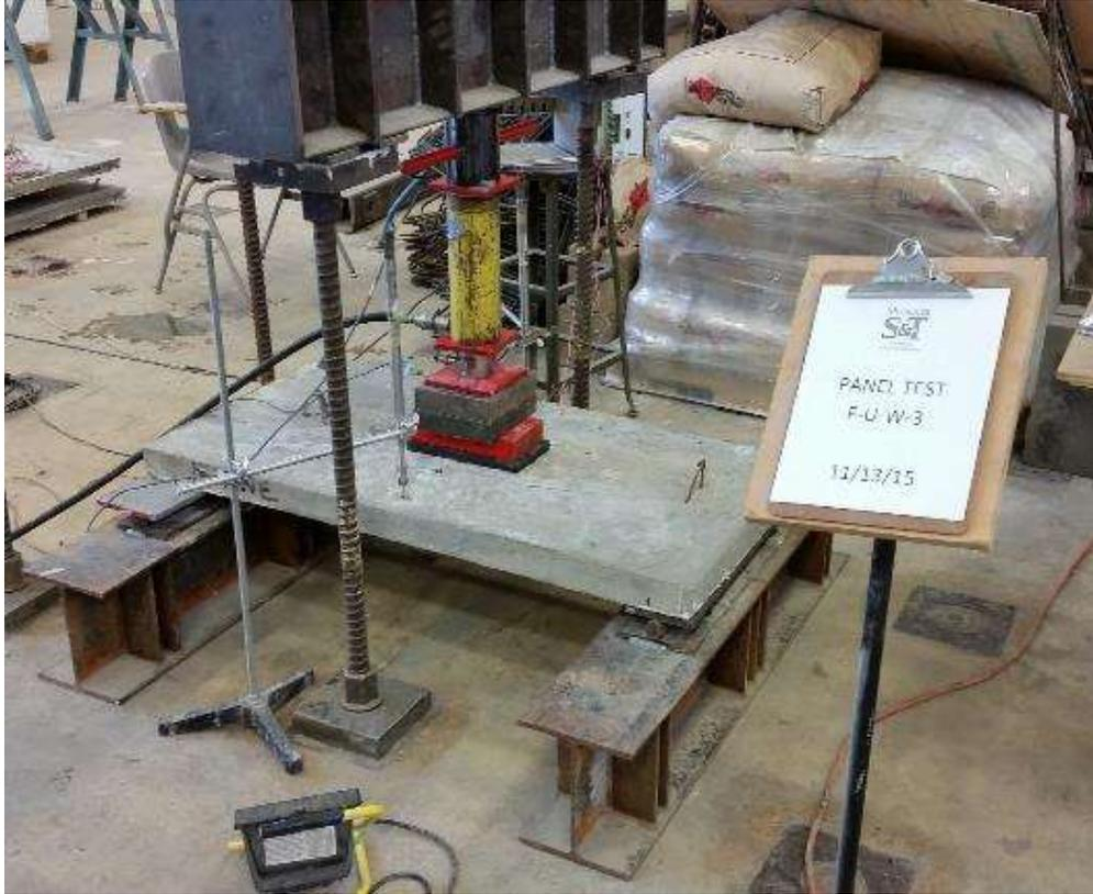
Figure 6.15. Panel FUW3 test setup
