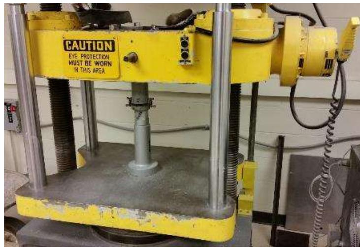
Figure 5.4. UHPC compressive strength setup
