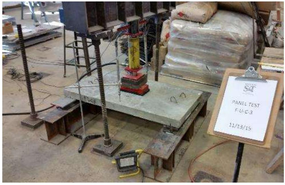
Figure 6.8. Panel FUC3 test setup
