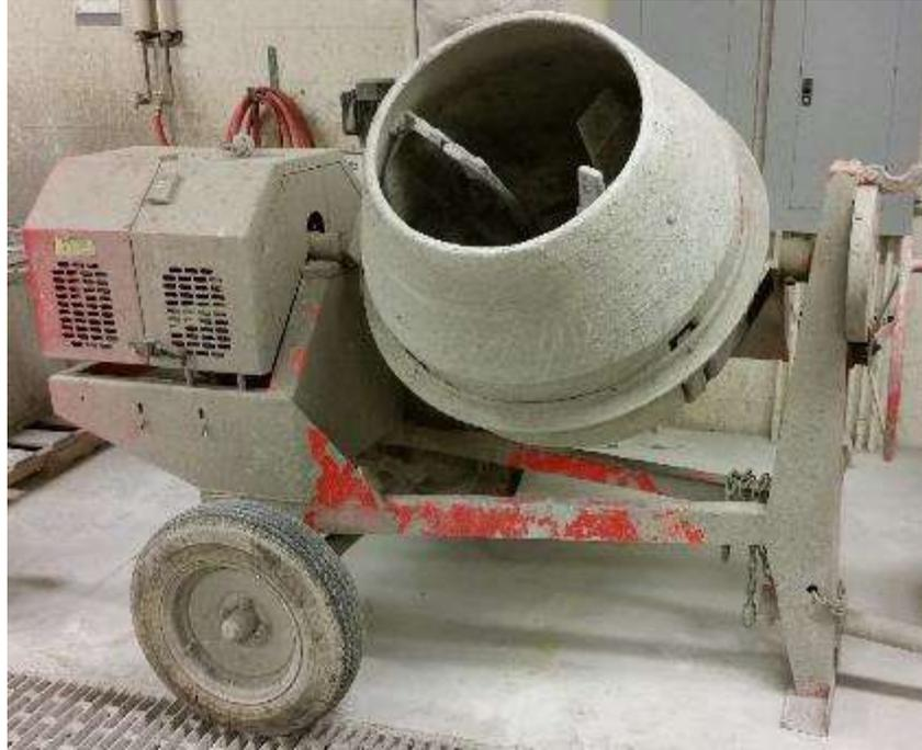
Figure 5.7. Conventional concrete mixer
