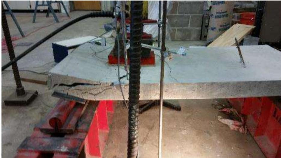
Figure 6.35. Diagonal tension failure on panel SCC3
