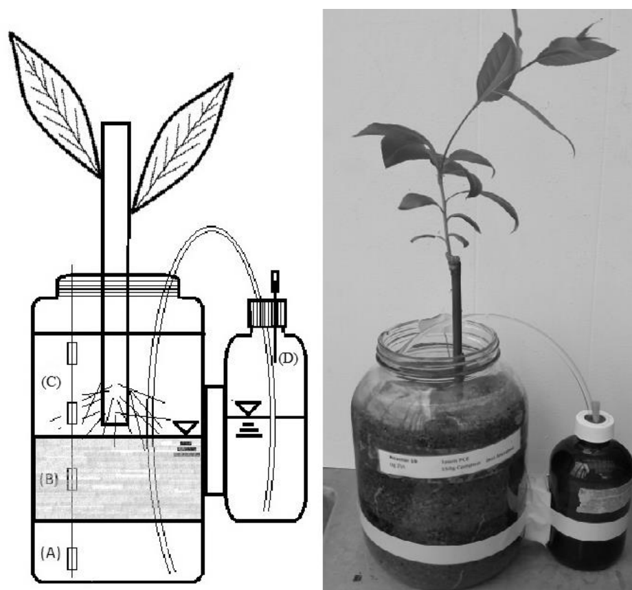
Figure 1 - Reactor Configuration Showing the Distribution Layer (A), Reactive Layer (B), and Rooting Zone (C). Dosing Bottle (D) was Connected via Siphon to the Reactor
