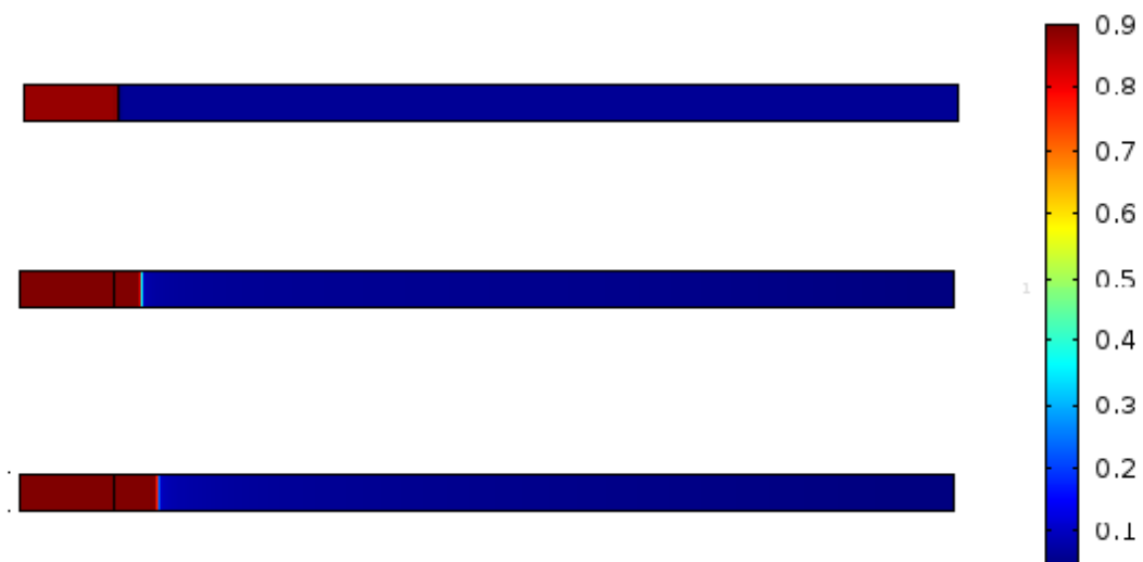
Figure 6.8. Concentration profiles at t=0 (top), t=0.808\text{s} (middle) and t=1.616\text{s} (bottom) for zero flux boundary condition for \phi=0.1\text{V}
