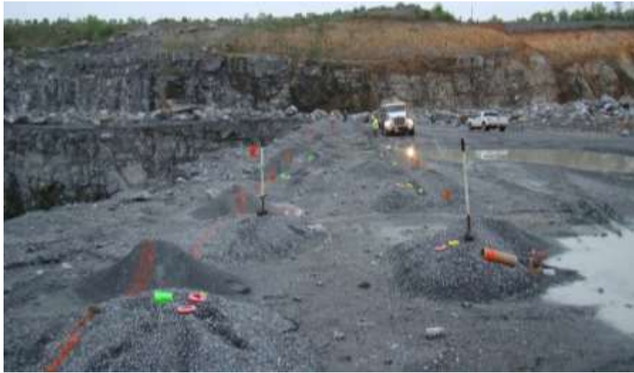
Figure 3.2. Hole Loading During Test Shot 1, with Titan 1000 SME Truck in Background
